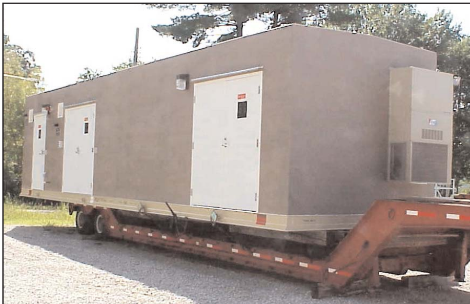
Chemical feed equipment in two compartments and finished station on trailer ready for shipment to site.
