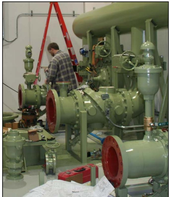
Shop assembly of mechanical components including pump check valves, isolation valves and the discharge header.
