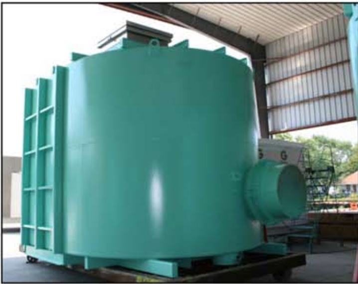
This picture shows the exterior of the finished 36" pressure reducing valve station ready for shipping.
